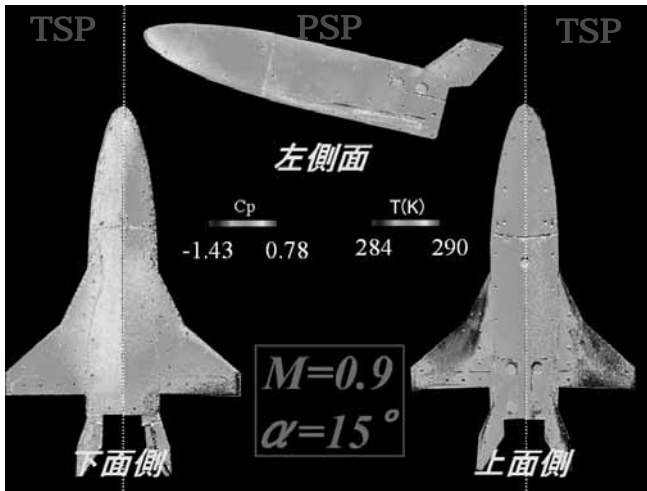
Fig. 7 Flow fields over the Shuttle model at M=0.9 , \alpha=15[deg] .
