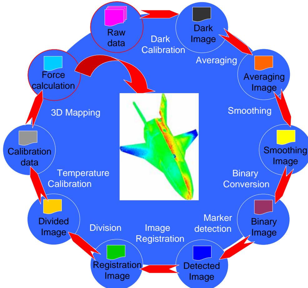
Fig. 1 Flow chart of image data processing of PSP measurement.
