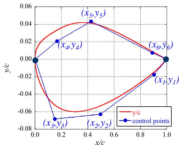
Fig. 1 B-Spline control points
